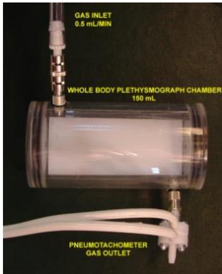
Figure 1. Custom made chamber for cylindrical chamber. By using the flat plastic insert, the final volume or dead space of the chamber is reduced to c. 150ml. The chamber has two ports: one for the gas inlet and one for the pneumotachometer (Hickey MM et al. 2010, Mosqueira et al 2013).
